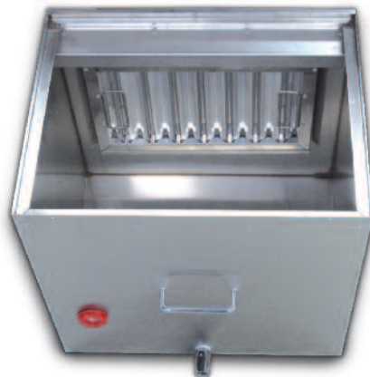
Aerosol separator fitted in front of the exhaust grid of the liquid collection tank
