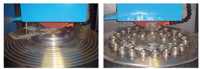
The face- and step-processing of flat rotationally symmetric work pieces is in many cases easier than with a classical cylindrical grinding machine. Especially heavy work pieces can easily be loaded and positioned onto the working table. Serial parts can be worked much economically as with a classical surface grinding machine, as the acceleration at the reverse points is not existent.
