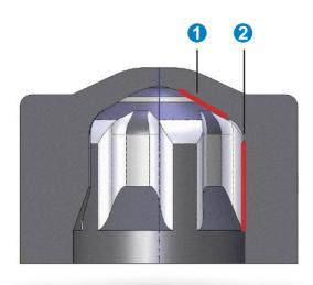
Grinding operations: 1 - seat, 2 - bore
